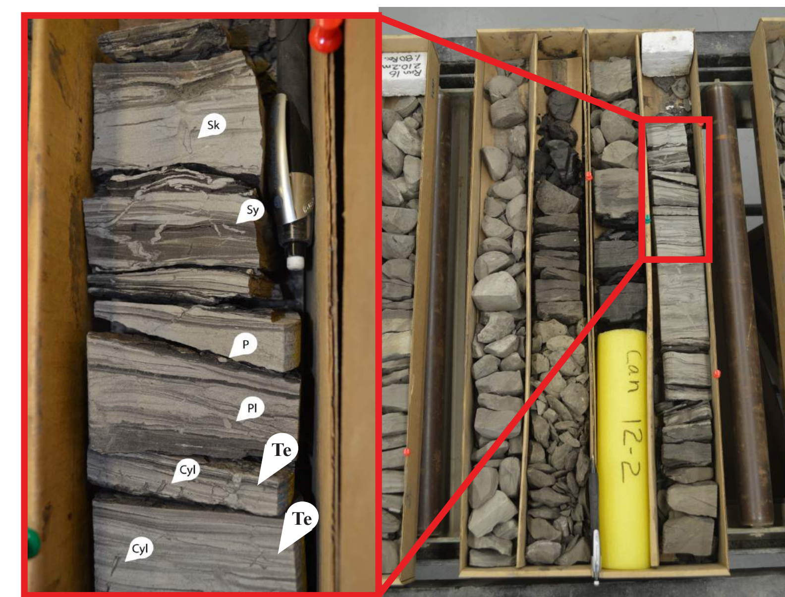
Figure 5. Core from 07-02-004-27W3. a) Photo taken directly below Bearpaw/DPF contact. Trace fossils and sedimentary structures suggest a marginal marine environment with brackish water. Coal seams and brackish water signatures commonly mark the transition to the overlying marine Bearpaw Formation in the Cypress Hills. Cy. Cylindrichnus P. Planolites ; Pl. Paleophycus ; Te. Teichichnus ; Sk. Skolithos ; Sy. Syneresis Cracks.
