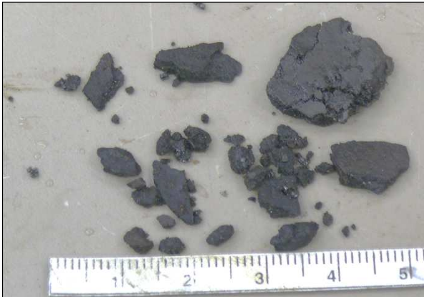
FIGURE 34 SCALE SAMPLE COLLECTED FROM INTERNAL SURFACE OF BUCKLE
