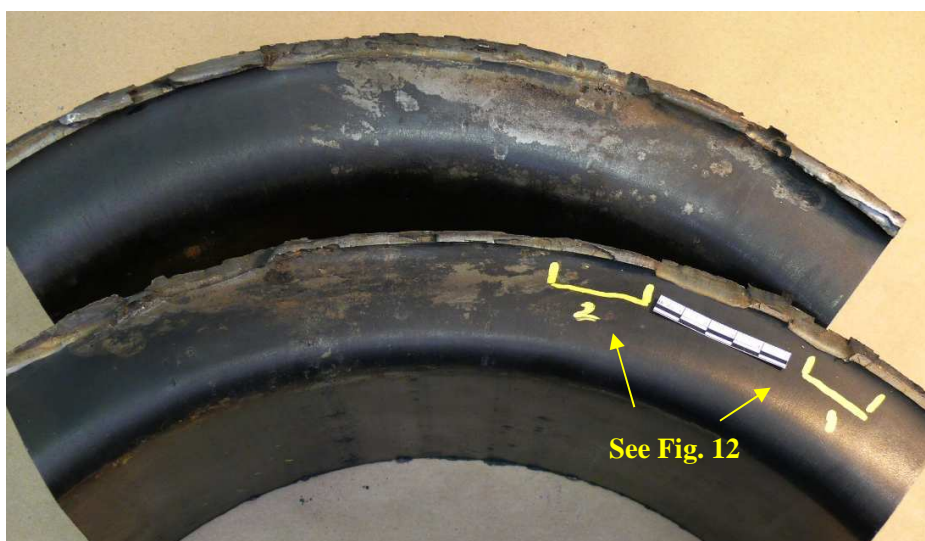
FIGURE 11 DEGREASED FRACTURE SURFACES
