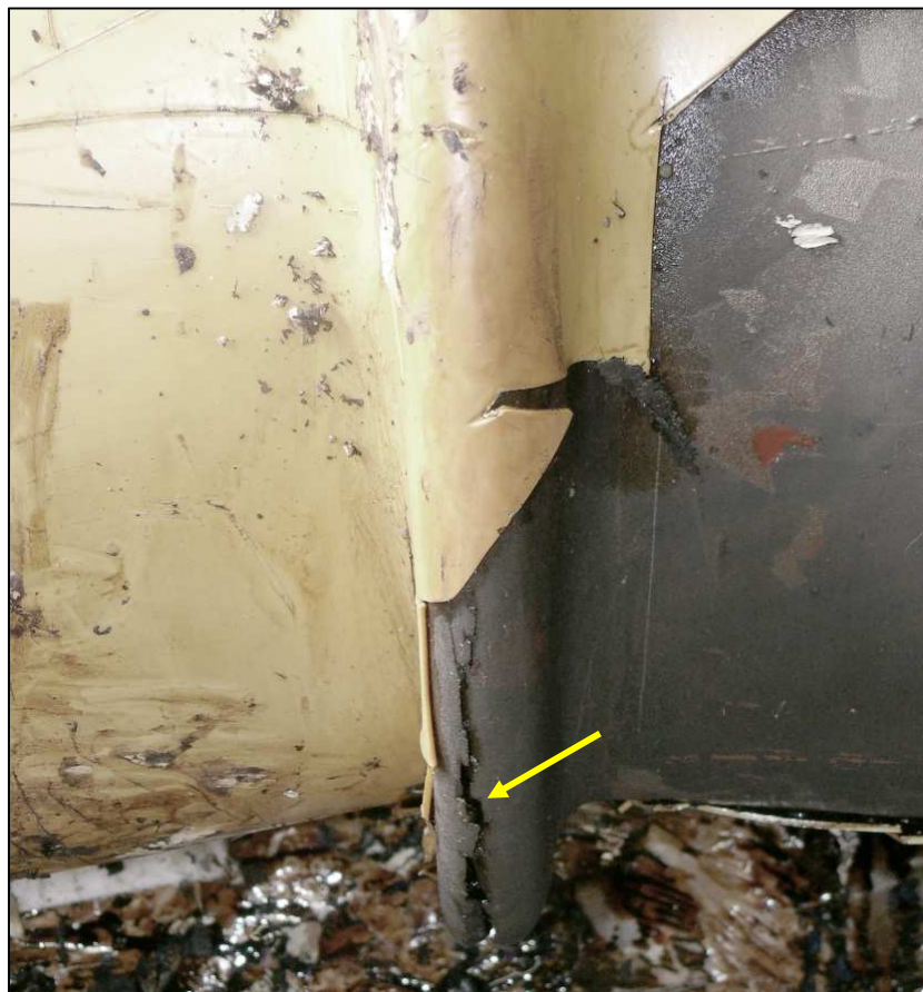
FIGURE 6 BUCKLE AND THROUGH-WALL FRACTURE AFTER CLEANING OD SURFACE WITH VARSOL
