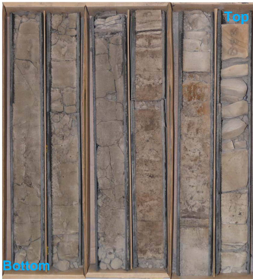
Figure 3 – Facies Association 1: Core box photograph of Facies 1a in well 13-01-052-27W3 core (487 to 482.5 m). Facies 1a is characterized by sandy mudstone with pervasive bioturbation (BI 3 to 5).
