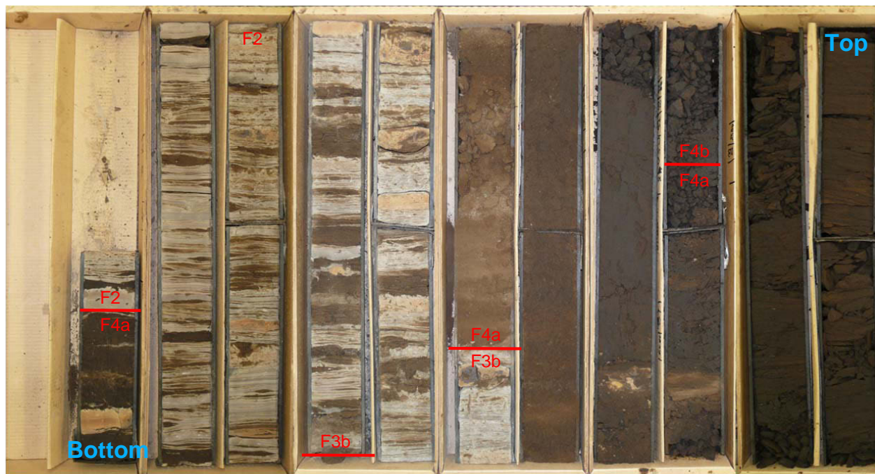
Figure 5 – Facies Association 3: Core box photograph of well 11-03-051-22W3 core (492 to 484.1 m) depicting the contact with Facies 4a and overall coarsening- and shallowing-upward successions of distal prodelta (Facies 2) to proximal delta front (Facies 4b). Note that Facies 4b is characterized by abundant current-rippled and small-scale trough cross-bedded sandstone.
