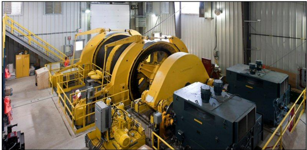
Figure 9:4 Typical double drum hoist installation
