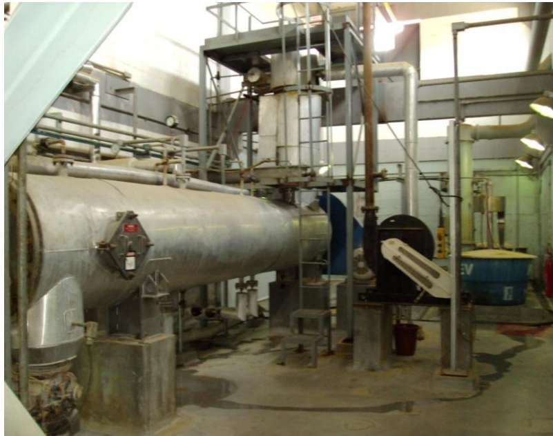
Figure 11:16 Uranium yellowcake dryer
