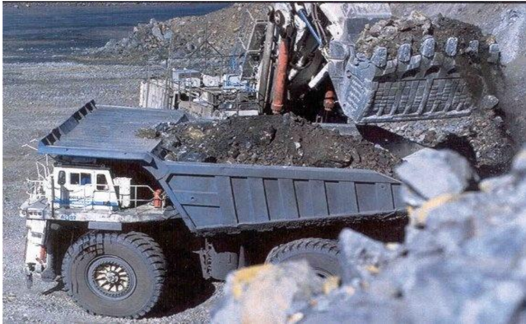
Figure 9:10 Excavator loading a haulage truck
