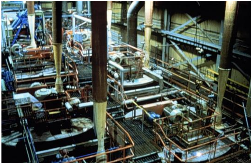
Figure 11:11 Uranium leach equipment, atmospheric pressure agitated leach tanks
