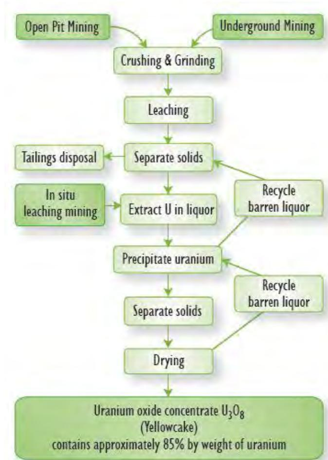
Figure 19: Simplified Uranium Mine Process Flow Chart
