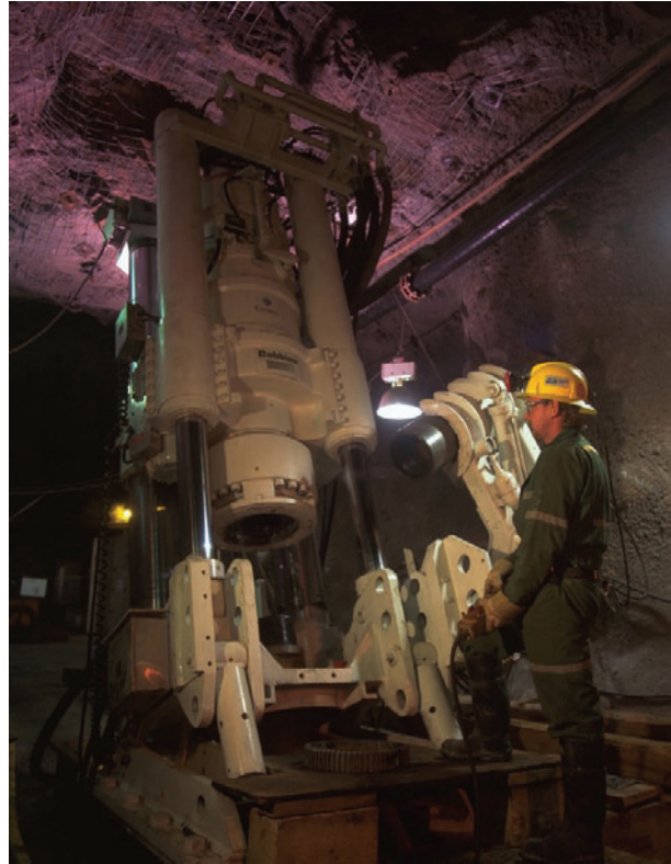
Figure 5 - Drilling a raise-bore pilot hole at McArthur River Mine. Photo courtesy of Cameco Corporation.
