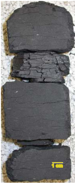
Figure 5 - Core from Nexen Battle Creek West 7-2-4-27W3; Belly River coal; depth 235.2 to 235.4 m.
