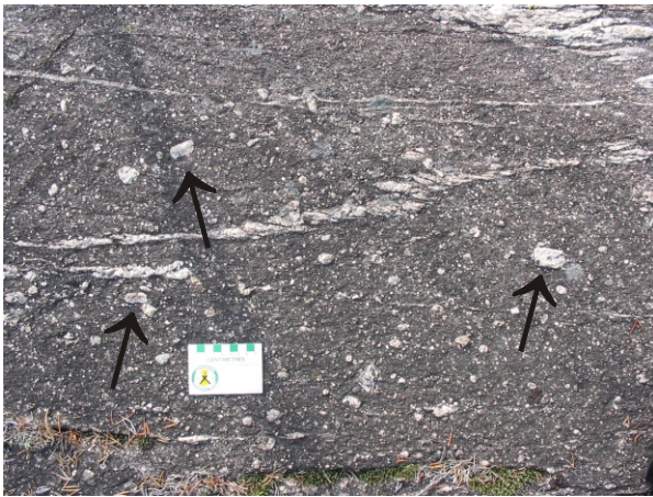
Figure 34 - Euhedral plagioclase phenocrysts (arrows) up to 3 cm long in tonalite; from west of Thompson Bay, Harper Lake (UTM 563287 m E, 6615756 m N).
