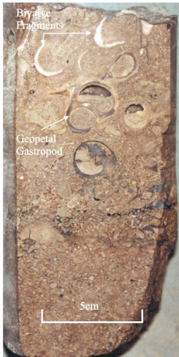
Figure 6 - Photograph of fossiliferous peloidal wackestones and packstones (lithofacies b) showing bivalve and coral fragments and a geopetal gastropod, from location 1-29-4-4W2 (1408.6 m).
