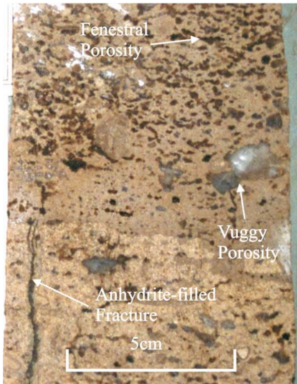
Figure 7 - Photograph of fossiliferous peloidal wackestone and packstone (lithofacies b) showing fenestral and vuggy porosity, and an anhydrite-filled fracture, from location 15-20-4-4W2 (1390.7 m).
