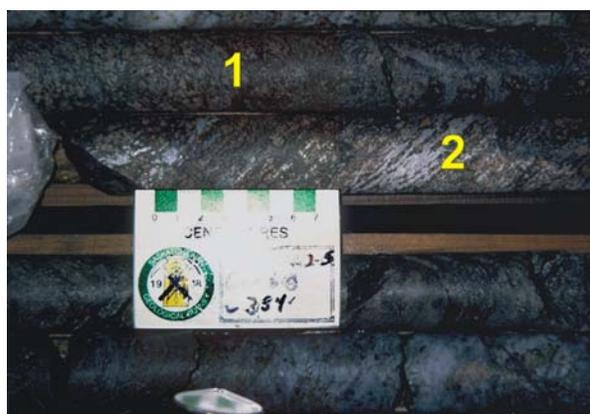
Figure 8 - Silicate-facies iron formation (1) containing 35 to 40% garnet porphyroblasts and a dark amphibole(?). Note the interlayered siliceous bands (2) interpreted to be primary chert layers (Car 60).
