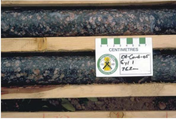
**Figure 5 - K-feldspar-phyric granodiorite from the Firebag Domain. Note the relatively homogeneous appearance when compared to granodioritic gneiss (Figures 7 and 11 below).**
