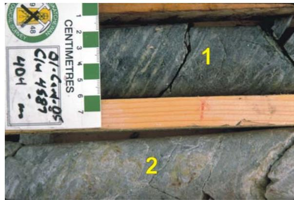
**Figure 12 - Mylonitic granodioritic gneiss (1) and massive granite (2). This mylonite zone is common at the transition between the Peter River gneiss and Earl River Complex (Clu 4587).**
