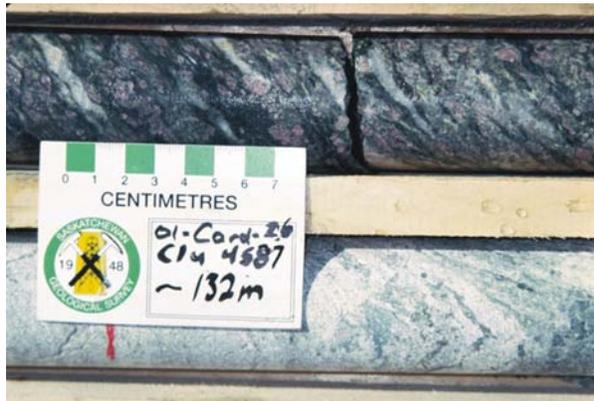
**Figure 10 - Garnet-cordierite migmatite is the dominant component of the Peter River gneiss. Note the large garnet porphyroblasts (Clu 4587).**
