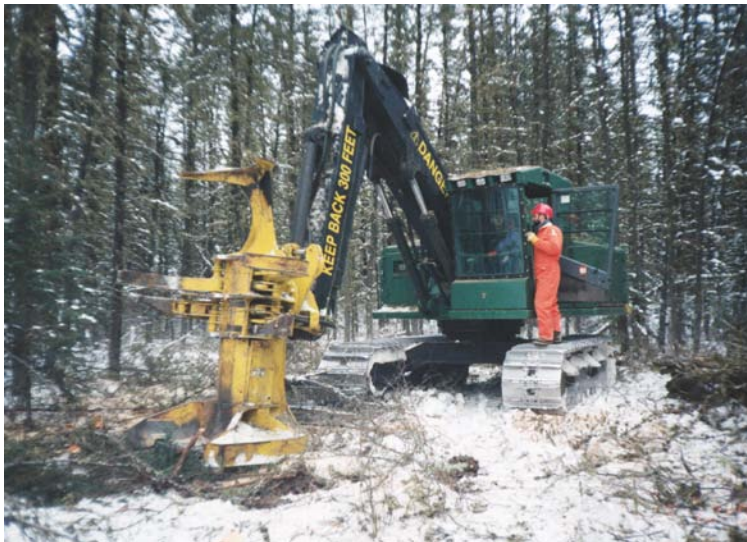
Figure 5. A mechanical harvester preparing to thin a softwood stand, Jeanette Lake Fuel Management Project.
