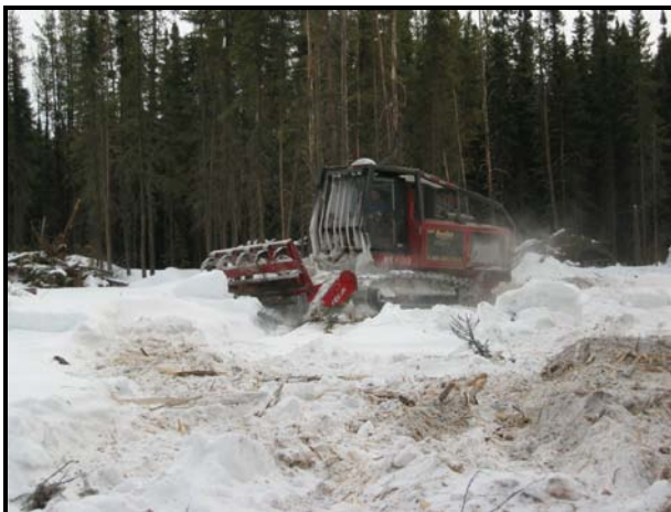
Mulcher at work on one of the piles of slash left after thinning work.
