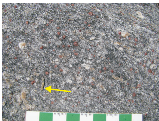
Figure 6 - Close up of migmatitic pelite with abundant garnet and sillimanite (arrow); station RM08-08-ST11-PH3 on south shore of Wunehikun Bay at UTM 645676 m E, 6116919 m N.
