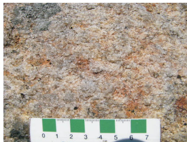
Figure 16 - Close-up view of orange-weathering, sillimanite-bearing quartzite; station RM08-37-ST14 near north end of map area at UTM 686916 m E, 6140483 m N.
