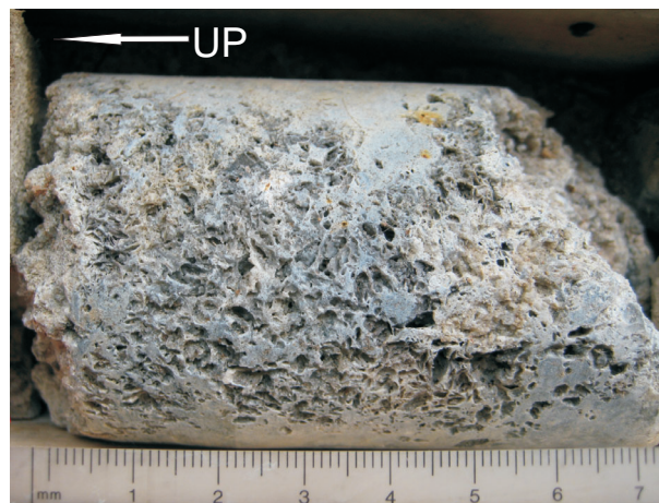
Figure 7 - Silicified marker unit at top of Success Formation in drill hole BD-09-10 at 57.0 m depth.
