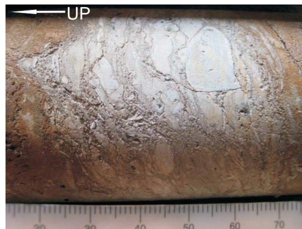
Figure 6 - Breccia texture in Success Formation in drill hole BD-09-13 at 137.8 m depth.
