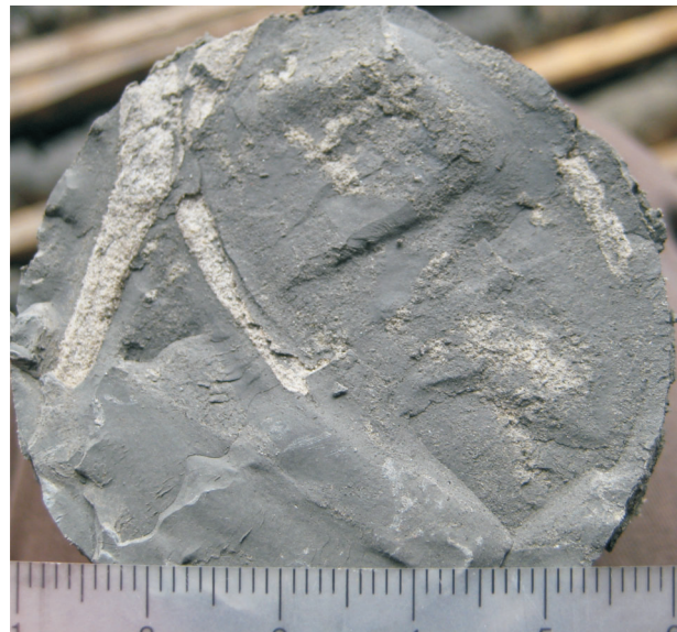
Figure 3 - Siltstone-filled burrows in Joli Fou Formation shale in drill hole BD-08-06A at 63.7 m depth. Scale card in centimetres.
