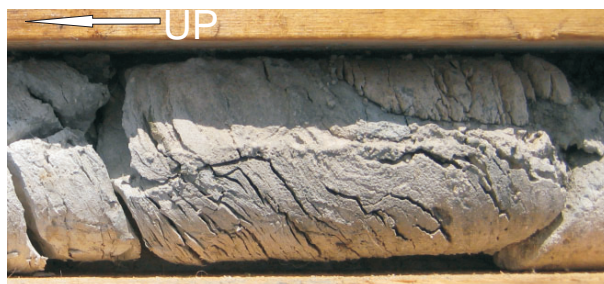
Figure 5 - Slumped texture in Success Formation in drill hole BD-09-27 at 133.5 m depth. The drill core is approximately 5.8 cm in diameter.
