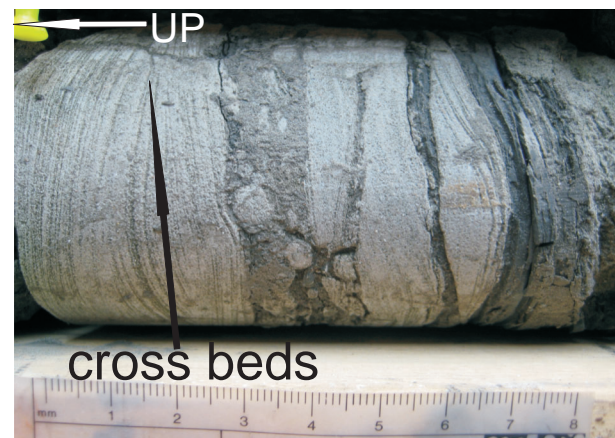
Figure 4 - Carbonate cemented cross beds at top of Spinney Hill Member in drill hole BD-09-24.
