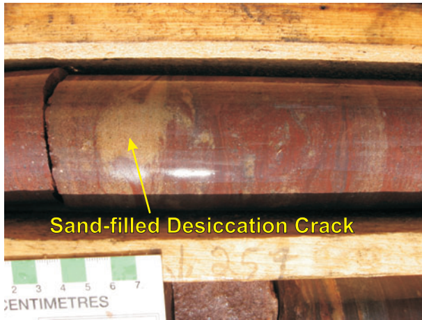
Figure 5 - Large desiccation cracks in red siltstone and mudstone filled with quartz sand at ~255.5 m in drill hole CRE-007.
