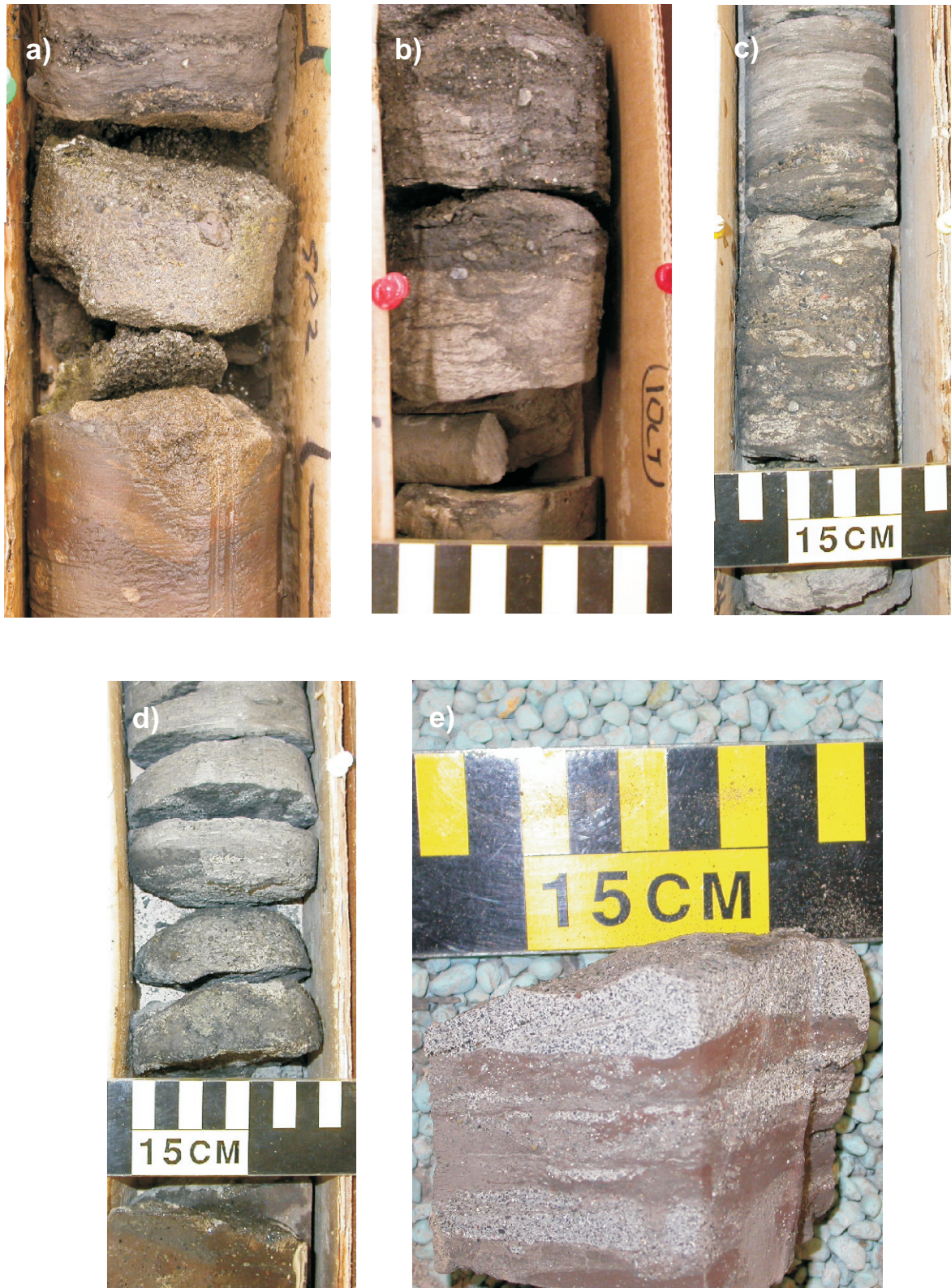
Figure 15 - Photographs of Viking transgressive lag: a) Gulf Totnes 31/11-17-28-18W3, pyritized chert-pebble conglomerate with scour surface into sideritized mudstone, 718 to 718.1 m; b) Ish Kindersley 01/6-35-28-24W3, bioturbated muddy sandstone truncated and overlain by pebbly mudstones, 710.5 m; c) NCO Plato N 01/10-15-27-19W3, bioturbated, multi-coloured chert pebble mudstone, 696.5 m; d) Murphy et al Kindersley 01/7-19-28-21W3, sideritized chert-pebble mudstone rip-up clasts, 743.5 m; e) Canus et al N Verendrye, 01/12-32-28-23W3, chert-pebble sandstone interbedded with sideritized mudstone, 2300 ft (701.04 m) (core diameters are in the range 7 to 8.5 cm).
