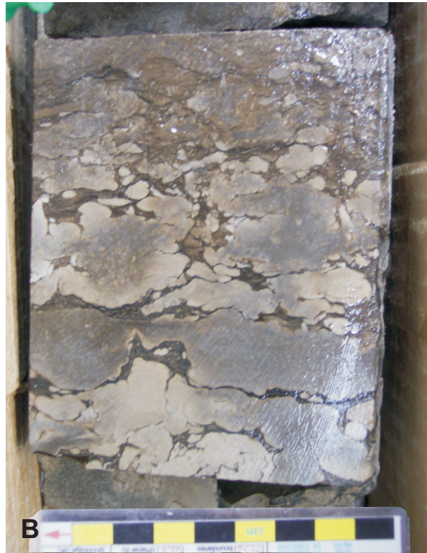
Figure 11 - Two types of mottling textures observed at the top of Facies Assemblage 1 in the Coronach Member. A) Faint mottled texture produced from rare light brown dolomite nodules (D) within a dark brown limestone matrix. Sample from 8-16-2-14W2 at 3020 m. B) High-relief, grey to beige dolomitic nodules within sparse limestone matrix. Sample from 11-20-2-18W2, 2994.9 to 2994.8 m.
