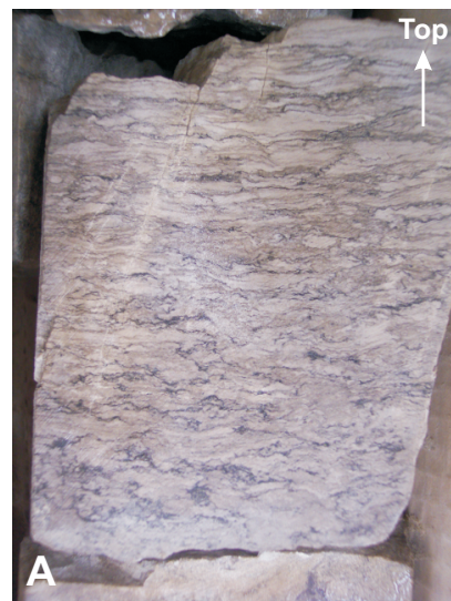
Figure 10 - Variations in fabric of the laminite facies. Basal, discontinuous laminations (A) grade up to irregular or "wispy" laminations (B) which grade up to sub-horizontal, more consistent laminations (C). Oil staining and fluorescence are best seen in laminites exhibiting textures like those in 'A'. Samples from 8-16-2-14W2 at depths of 3018 m, 3016.6 m, and 3016.2 m, respectively.
