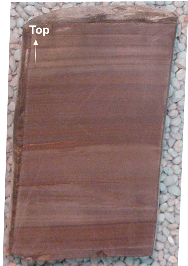
Figure 4 - Black, organic-rich, horizontal laminites from the base of Facies Assemblage 2. This facies has a very strong petroliferous odour and is a potential source rock in the Coronach Member. Sample is 9 cm wide, from well 12-2-7-11W2, 2548.05 to 2547.9 m.
