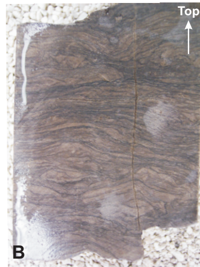
Figure 9 - Top of Facies Assemblage 1 marked by sharp, irregular contact, probably an erosional surface. Below contact are small laminar labechiid stromatoporoids ('S'; B. Pratt, pers. comm., 2007) and sediment-filled Planolites (P) and, possibly, Teichichnus burrows (T). Contact is overlain by cross-laminated grainstone. Sample from 8-16-2-14W2, 3019 m.
