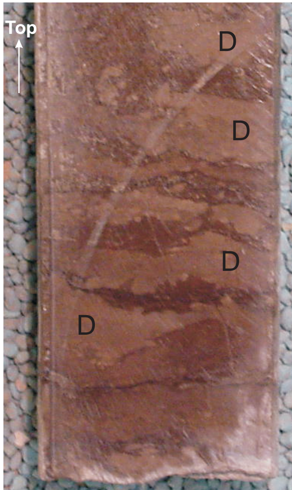
Figure 3 - Mottled texture from light brown dolomite nodules (D) in a dark brown limestone matrix. Core is 9 cm wide. Sample from 12-2-7-11W2, 2550.4 to 2550.2 m.
