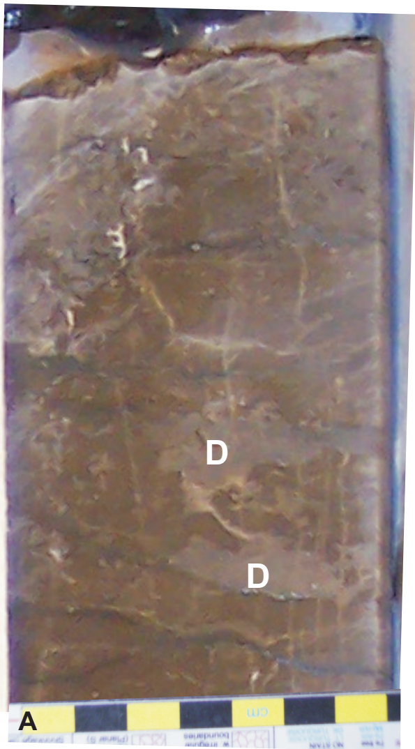
Figure 11 - Two types of mottling textures observed at the top of Facies Assemblage 1 in the Coronach Member. A) Faint mottled texture produced from rare light brown dolomite nodules (D) within a dark brown limestone matrix. Sample from 8-16-2-14W2 at 3020 m. B) High-relief, grey to beige dolomitic nodules within sparse limestone matrix. Sample from 11-20-2-18W2, 2994.9 to 2994.8 m.
