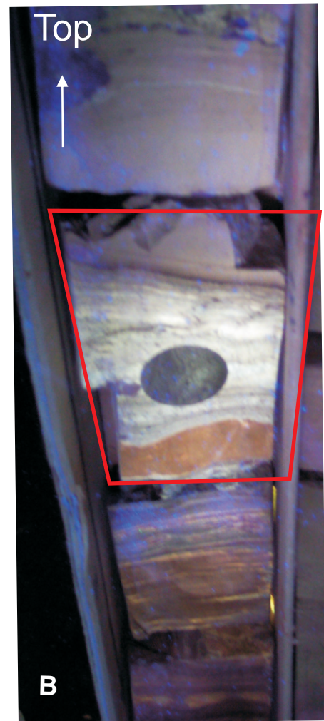
Figure 5 - A) Top of laminite facies (from Assemblage 2) showing displacement of laminations due to growth of nodular anhydrite. Facies has a sharp, 15° angle contact with tight massive dolomudstones above (Assemblage 3). Sample from 12-2-7-11W2, 2546.95 to 2546.8 m. Core is 9 cm wide. B) The same sample (outlined by red box) under UV light showing bright yellow to orange fluorescence in laminite facies.
