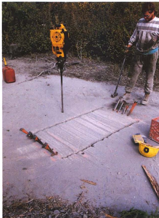
Unexpected strength parallel to foliation make sampling difficult.
