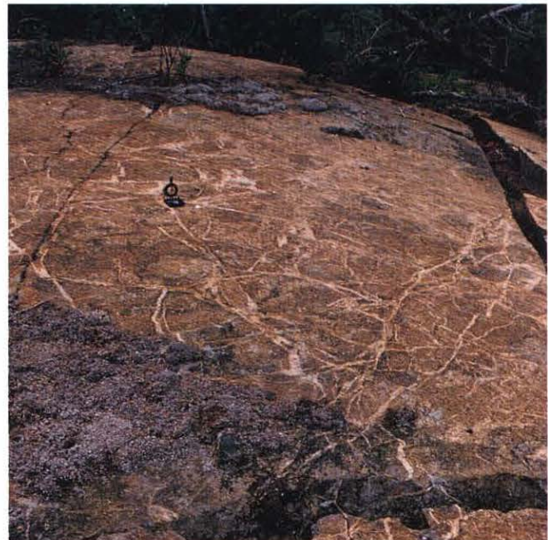
Compact dolomite (top) and metadiorite (bottom) are termed “marble” in the trade.
