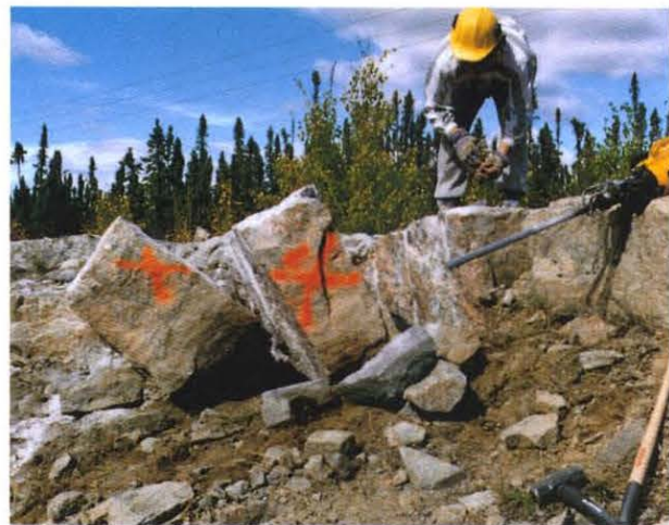
Sahli Granite splits readily along a planar “grain” direction - an excellent quarrying feature.
