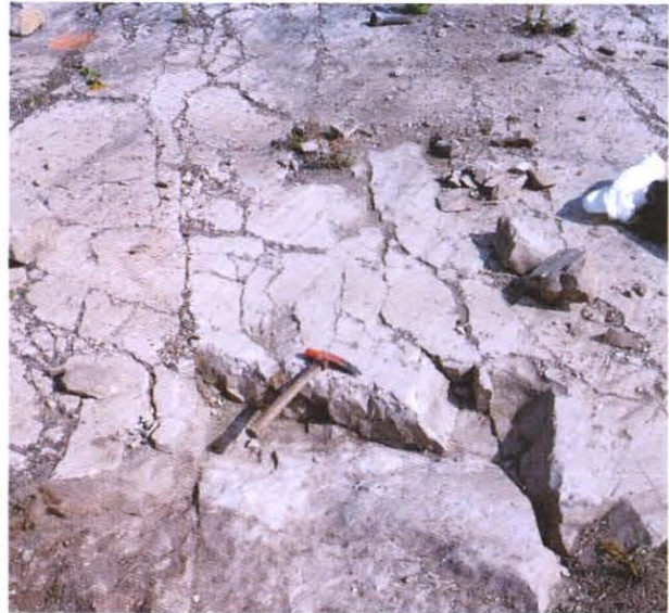
Most minor fractures on the marble surface end on a horizontal spall.
