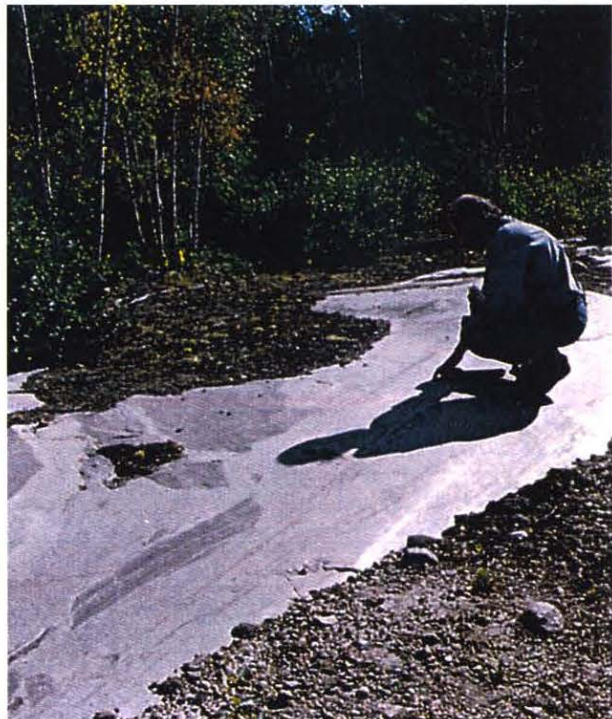
Lack of uniformity disqualifies this otherwise sound stone.
