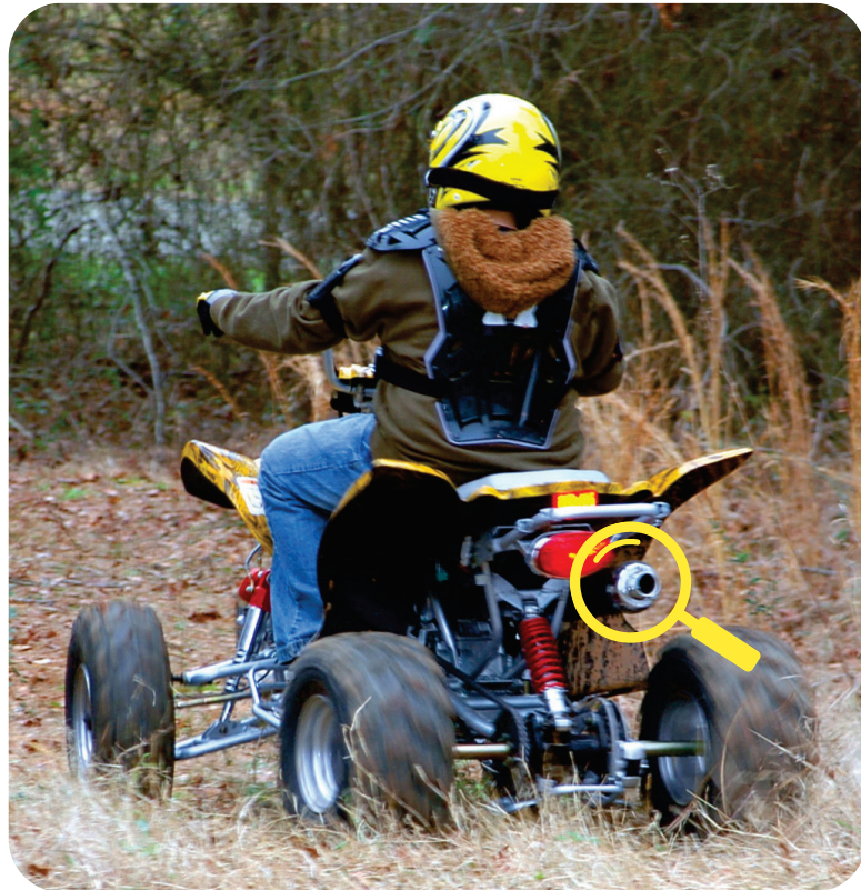
Exhaust pipe with a spark arrestor
