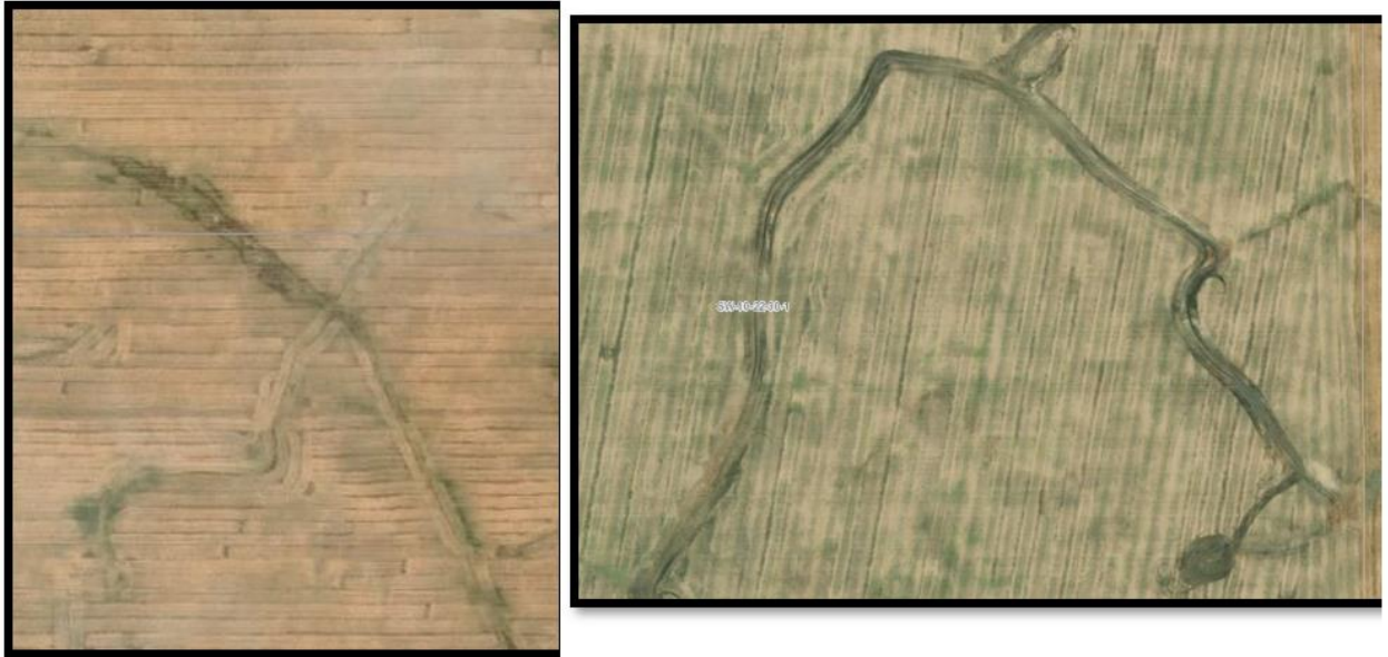
Figure 10: Constructed surface ditches provide a hydrological connection from a potentially impacted site to a permanent waterbody
