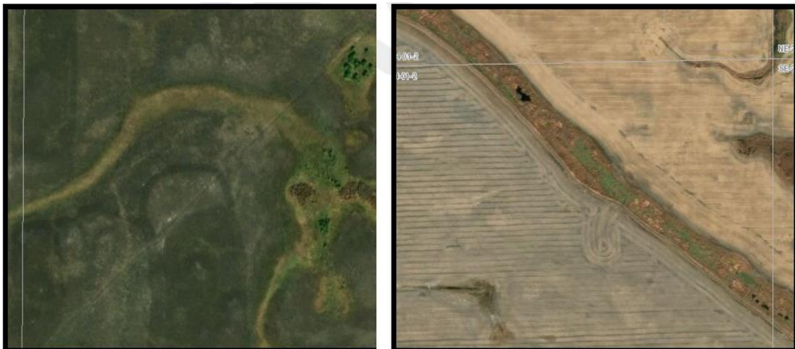
Figure 9: Continuous liner stream features indicate a hydrological connection from a potentially impacted site to a permanent waterbody
