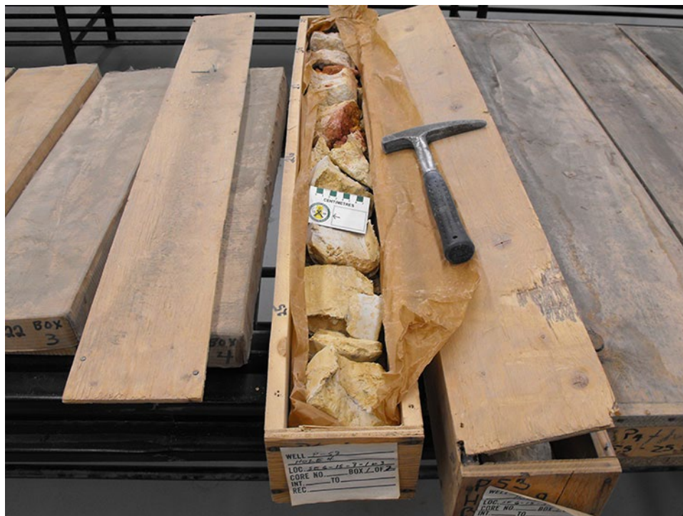
Figure 5 – Drillhole Rockglen Stoneware Clay P53 Hole 4 core, showing the anomalous REE-bearing sample CL-21-2019 taken from white, relatively pure, massive kaolin clay in interval 7.47 to 8.84 m of the Ravenscrag Formation Willow Bunch Member.
