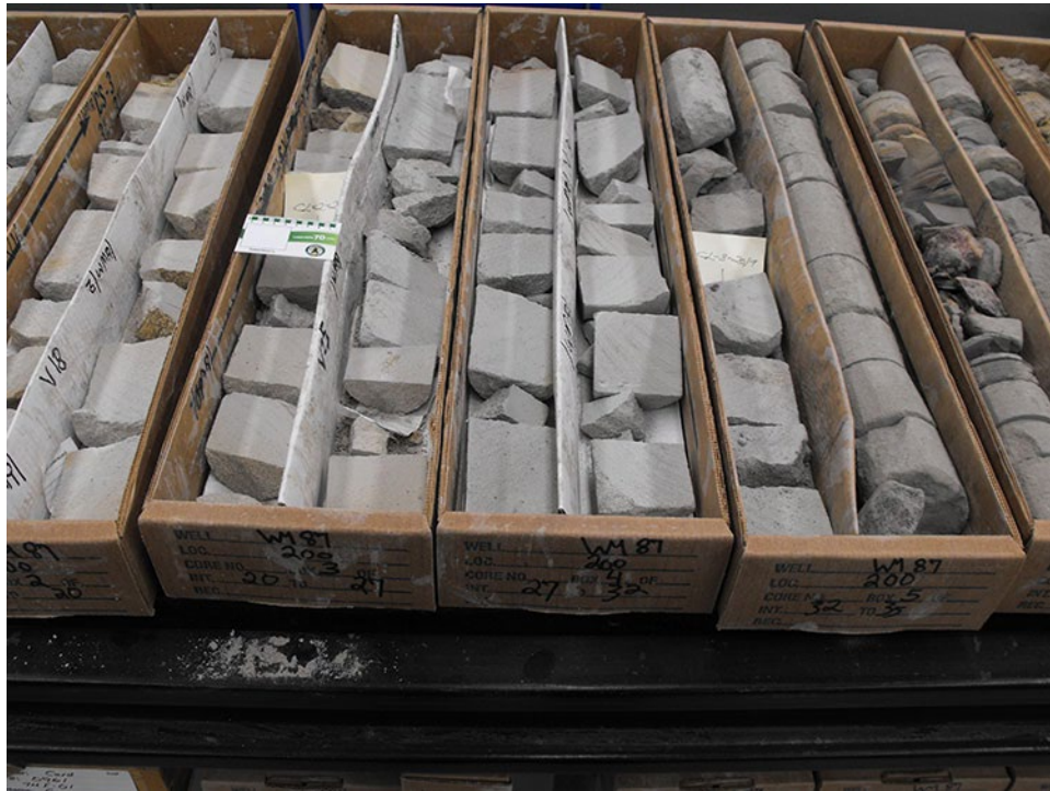
Figure 3 – Drillhole Ekaton Project 12 Kaolin WM87-200, large diameter (7 cm) core of an Upper Cretaceous Whitemud Formation kaolin interval. Note the sample intervals for this project, marked by yellow, labelled paper. This core was previously split and sampled during the original drilling program in 1987 by Ekaton Industries Inc.
