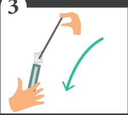
3 Using a pushing stick, insert the screens gently into the stem
