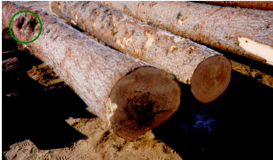
Figure 18 External Indication of Rot in a White Spruce Log
