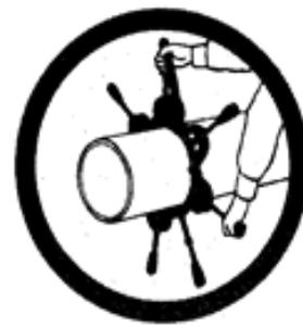
Cutting asbestos-containing pipe by hand.
