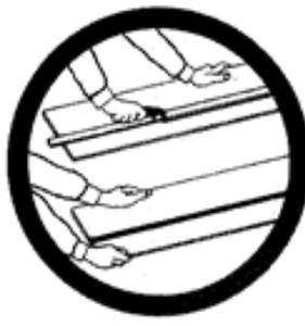
Cutting asbestos-containing wall board by hand.
