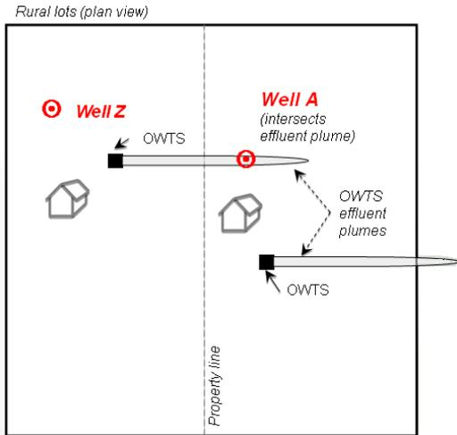
A well intercepting a plume occurs when treated effluent is drawn into the well as shown below for well B and well C. Well A in the diagram below intersects a plume but does not intercept it.
