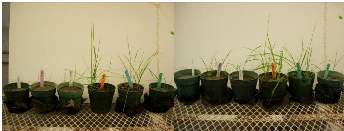
Photo 4. Elymus innovatus (hairy wild rye) grown in Orion (left) and Star (right) fine processed kimberlites. Treatments from left to right in each photo are unamended, sand amended, agricultural soil, biosolids compost, yard compost, inorganic fertilizer.
